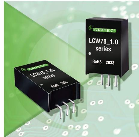
The LCW78\_1.0 series is a non-isolated POL switching regulator with an ultra-wide 14:1 high input voltage range (5-72VDC) with 1A output current that comes in a standard SIP3 package, covering most of the battery ranges and the standard power bus. This series offers high efficiency up to 96% and a very low quiescent current: 500uA.
